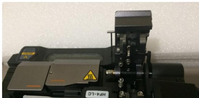
disposal bin. If necessary, use tweezers to pick up glass remnants and place in bin. Try to avoid sweeping glass remnants into the cleaver machinery to prevent interference; if needed, use a swab and cleaning fluid to draw out material from cleaver assembly.
