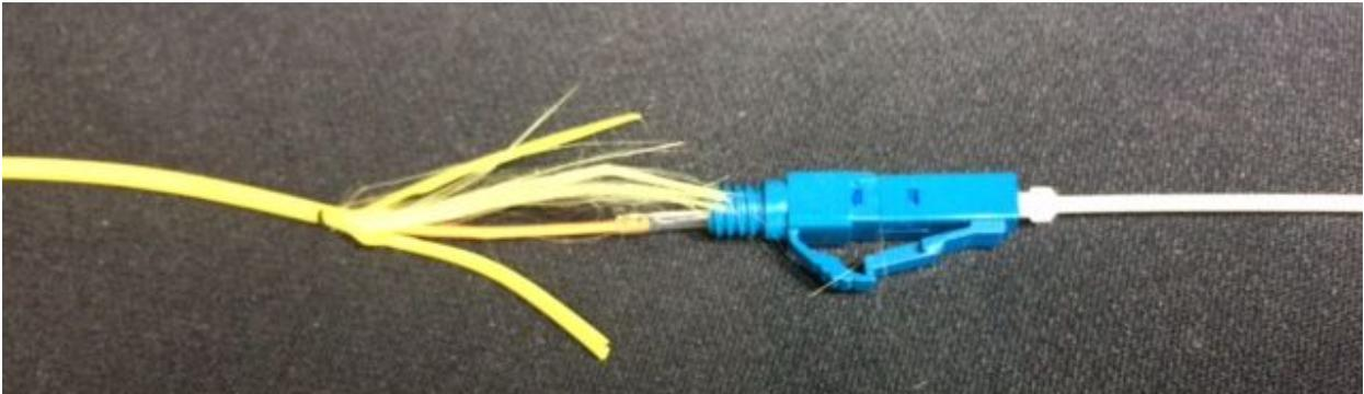
12. Next, the white screw-on cap is slid up past the jacket halves BUT ALLOWING THE KEVLAR TO REMAIN INSIDE IT. If the Kevlar slips out, it needs to be threaded through the white cap. Ensure the Kevlar is captured between the threads of the white cap and the rear housing. If necessary, loosen the cap and trim any Kevlar that extends outward.
