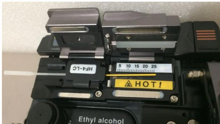
7. Using a lint free wipe and cleaning fluid, carefully wipe the exposed fiber to remove any remnants of coating.
