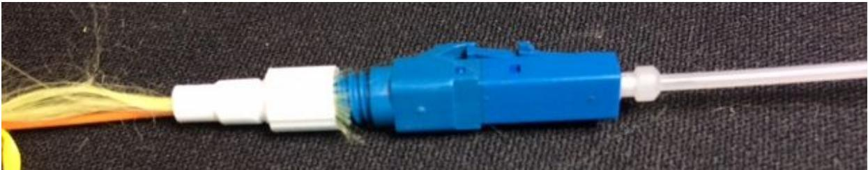
13. Place the jacket halves on either side of the white screw cap. Slide the heat-shrink tube up over the jacket halves onto the white cap.
