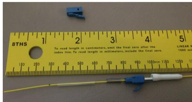
splice sleeve should be put onto the cable and slid to an appropriate spot away from the splicing process.
