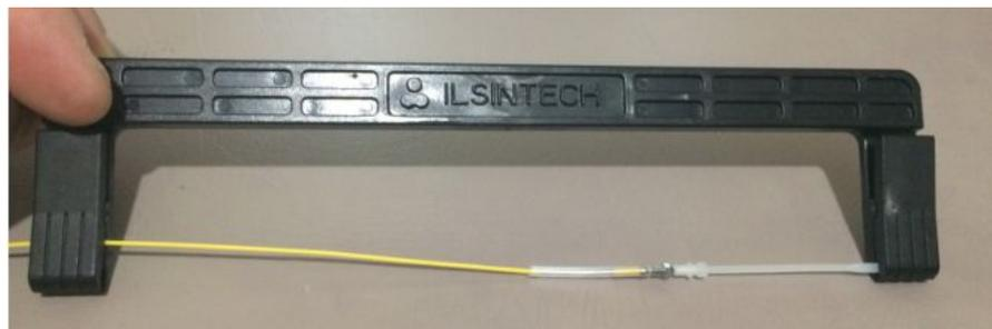
the LC connector is laying flat on its' base, with the anti-snag latch facing up toward the door of the heating chamber.
